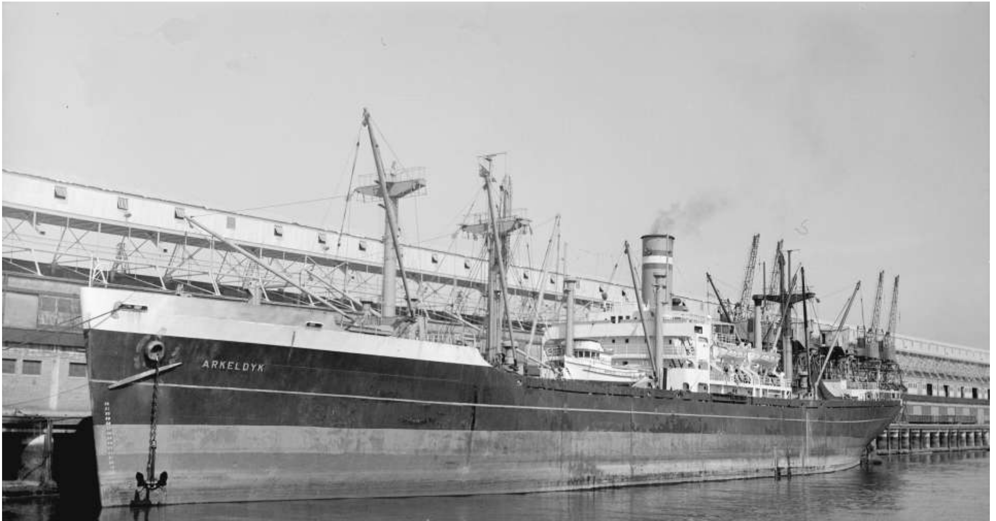
The more modern design of Victory ships like the ARKELDYK (the former WHITMAN VICTORY) with its slightly larger size and more powerful steam turbine engines ensured that they could travel in in high-speed convoys, making them more difficult targets for German submarines. On her foredeck is the GERONIMO, a wooden trawler brought up from Los Angeles at Ballantyne Pier on Tuesday, July 31, 1962 (Vancouver Archives, CVA 447-3308, Photographer - Walter E. Frost)
