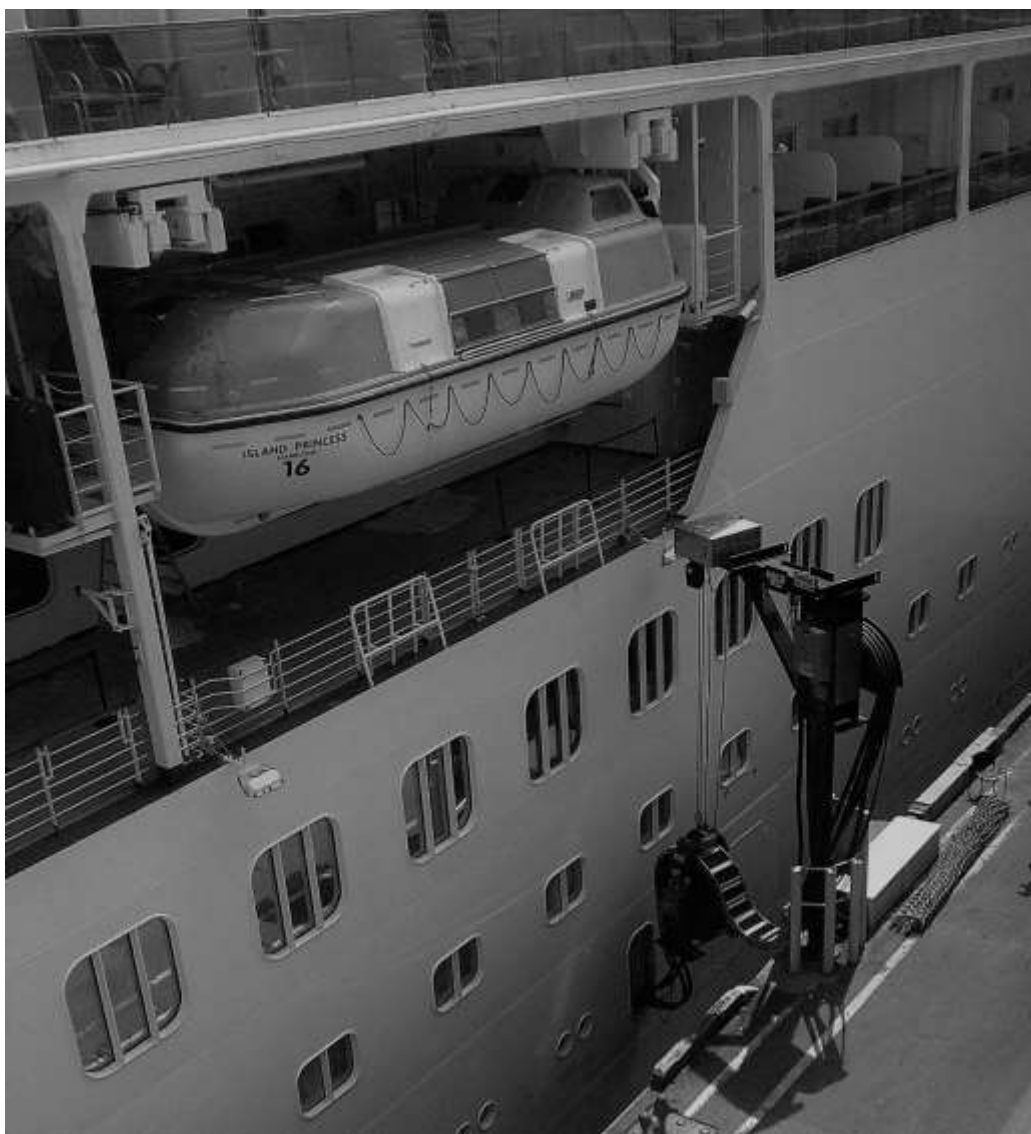
Canada Place's shore power jib providing land-based electrical power to the cruise ship MS Island Princess on July 4, 2012 (VFPA 038-3-9062)
